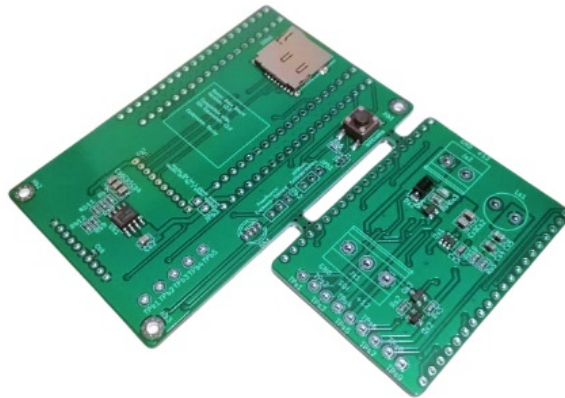
Figure 4.6: Second version of the PCB. These were purchased as a single board that could be snapped apart. No through-hole components have been soldered in this image.
